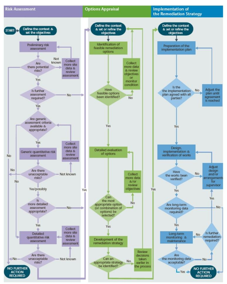
Note: The process may apply to one or more pollutant linkages each of which may follow a different route. For some linkages, it may be possible to stop at an early stage – others will progress all the way through the process. The level of complexity of each stage may also vary and in some cases may be very simple.
